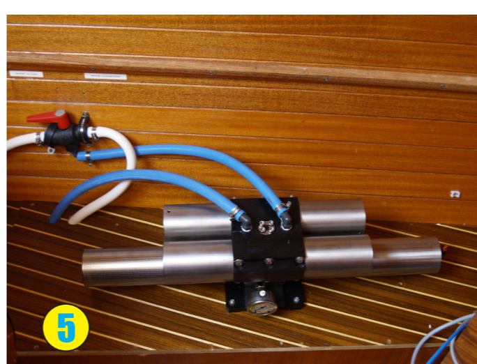
4. Pressure intensifier & membrane assembly bolted into position inside sofa.
